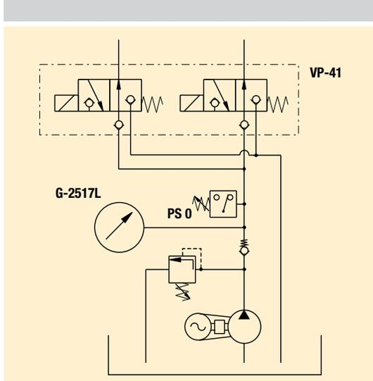
Pressure switch (PS 0) switches the motor off at maximum pressure; in case of pressure drop due to activating circuits, the motor restarts.
