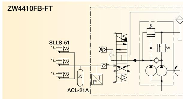
■ **ZW5410FB-FT** used to control clamping cycle on a horizontal machining center.
