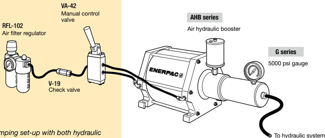
**I** In an automated clamping set-up with both hydraulic and pneumatic components, AHB series boosters are used as a power source for the hydraulic system.
