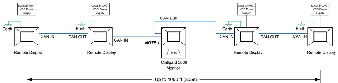
Fig. 10 Connecting four remote displays to a single Chillgard 5000 Monitor
