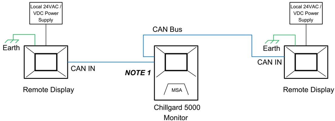
Fig. 8 Two remote displays using separate CAN bus runs
