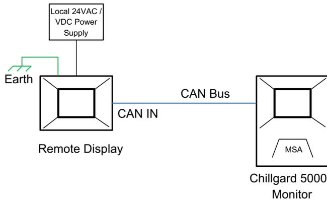
Fig. 7 Single remote display connection
