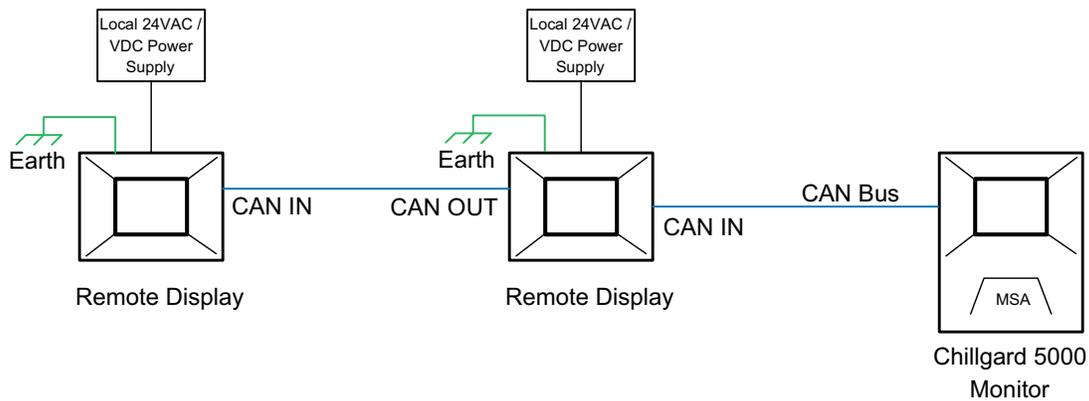
Fig. 9 Two remote displays using “Daisy Chain” configuration. CAN IN of the first remote display must be connected to the Chillgard 5000
