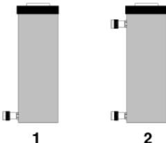
**IMPORTANT:** Double-acting cylinders must have both couplers connected.
