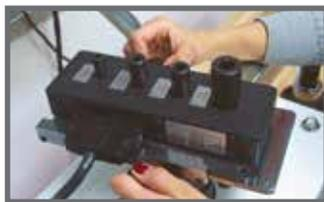
4 in 1 Transducer Kit with Mounting Adapter.
