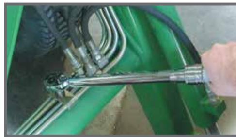
**MICROMETER ADJUSTABLE NEWTON METER TORQUE WRENCHES - SINGLE SCALE**
