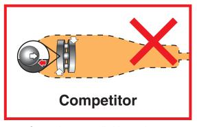
Competitor torque limiting tools use ball bearings or teeth to carry the torque load across the handle, wearing out the mechanism quickly.
