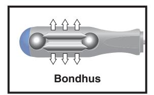
Bondhus ClickSet<sup>™</sup> Torque Limiting Screwdrivers distribute the torque load along the handle, redistributing force over a larger surface for greater accuracy and longer tool life.
